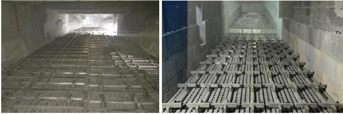
Figure 7. Illustration of cooler upgrade (before and after) planned for RK#1
