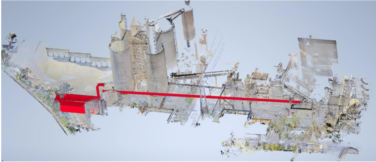
Figure 4. Schematics of RK#1 and the planned RDF feeding system in red
